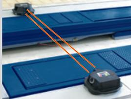
Can be used on any 4 post or scissors lift. Automatic lift level compensation.
