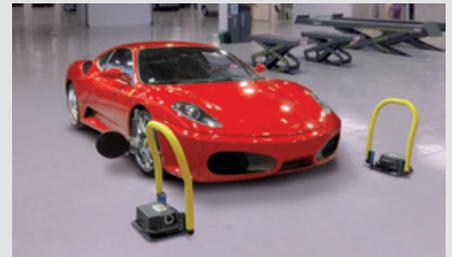
QC2R (Quick Control 2 Reverse) allows to quickly diagnose front axle angles: total toe and camber. After measurement the user will decide whether to carry on with alignment operation and vehicle adjustment.
